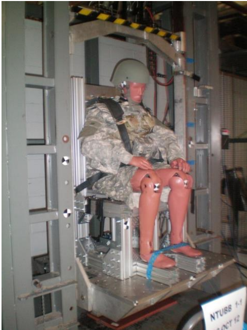
Figure 1: Vertical Drop Test Setup
